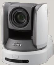
The BRC-Z700 offers a resolution of 1,040,000 effective pixels by deploying three 1/4-type ClearVid™ CMOS image sensors in combination with Sony-developed DSP technology. This camera includes a 20x optical auto-focus zoom lens with an optical image stabiliser. The perfect choice for long-distance-shooting applications, such as sporting coverage, this camera provides dual SD/HD outputs, enabling users to smoothly shift towards adopting a total HD system.
