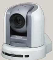
The standard-definition BRC-300 comes equipped with three 1/4.7-type Advanced HAD™ CCD sensors. This camera delivers dependable picture quality and is the best for cost-efficient SD applications. It can capture images in 4:3 and 16:9 aspect ratios, the latter providing a wider viewing angle.
