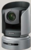
Equipped with three 1/3-type HD CCDs, the BRC-H700 offers excellent picture quality with high sensitivity and a high resolution of 1,070,000 effective pixels. This camera has the best sensitivity of the BRC Series; it therefore delivers superior performance in dimly lit environments, such as concert or wedding halls. Moreover, the camera offers the widest viewing angle of the BRC Series, delivering wider images of each scene and providing a complete picture of ongoing events.
