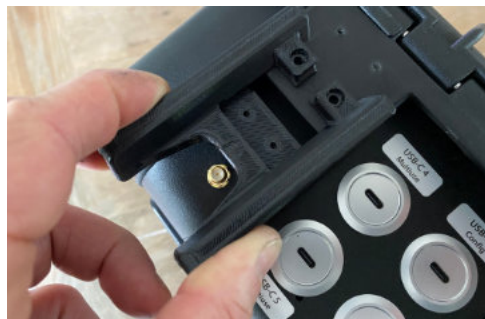
(Fig. 18) Slide the antenna protection into the designated pocket
