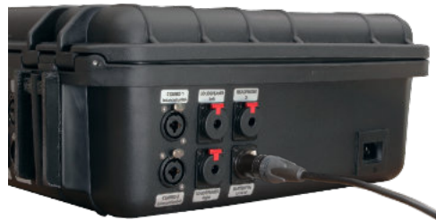
(Fig. 24) BSS case battery connection with attached adapter cable
