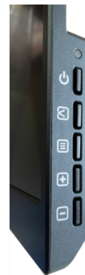
(Fig. 22) Control elements on the right side of the monitor
