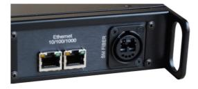
10/100/1000Mbps Base T for Ethernet, Full & Half Duplex 2 RJ45 ports works as a Switch Rear handles to protect connectors NO2-4FDW-A NEUTRIK as Optical Fiber Plug \*
