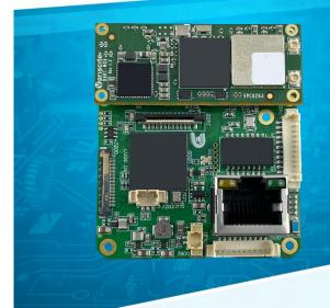
**Red Mamba Neo IP** video encoding module has been specifically designed for compact embedded vision systems.
